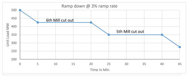
min as per stair-case curve given below. With block wise ramp down may be to tune of **75 MW per 15 min** time block. Similar way ramp up may also be possible at such rate.
