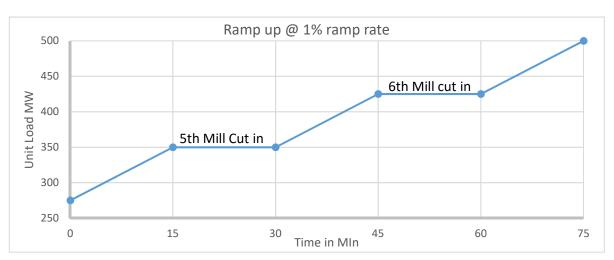
down operation. Hence achieving continuous load ramp rate from minimum load i.e. 55% till full load (100% load) and vice versa is difficult. The following graph shows practically achievable loads with 1% ramp rate while maintaining safe boiler operation.
